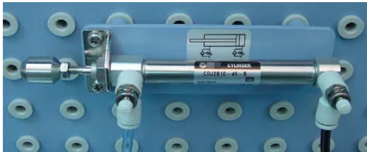
Figure 7 (a) Double-acting cylinder [13]. (b) Pneumatic symbol of a double-acting cylinder
