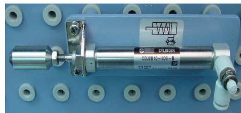
(b) Pneumatic symbol of a single-acting cylinder
