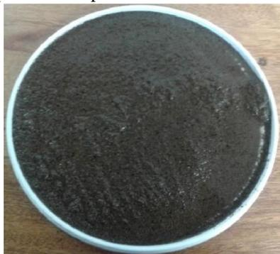
**Figure 1:** Activated sludge sample harvested from an anaerobic digester.
