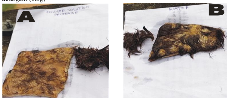
Figure 4A - B: Dehairing ability of alkaline protease produced by Bacillus tropicus PW10 -2 A2 on cow skin against the negative control. Key: A- Alkaline protease produced by Bacillus tropicus PW10 -2 A2; B - in sterilized water.
