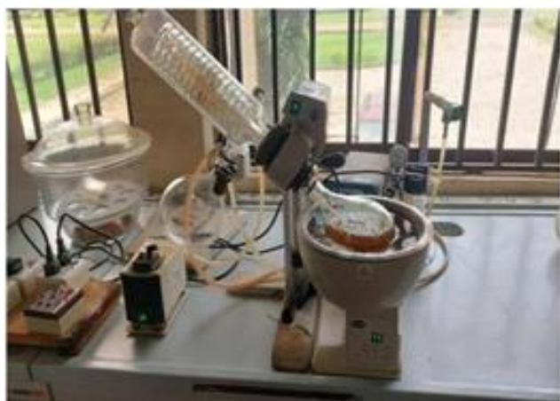
Figure 2: Rotary evaporator for separation of oil from solvent.
