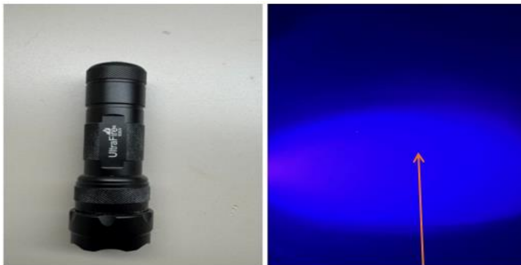
Figure 1: (a) Ultra Fire (395-405nm) handheld torch (b) Ultra Fire (395-405nm) handheld torch showing the emitted light beam used to enhance visibility of implanted monofilaments during localization.
